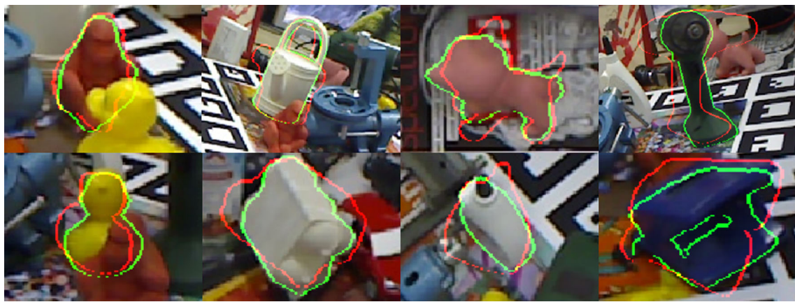
Fig. 8 Examples of refined poses on the Occlusion LILNEMOD dataset using the results from PoseCNN (Xiang et al. 2018) as initial poses. The red and green lines represent the silhouettes of the initial estimates and our refined poses, respectively (Color figure online)
